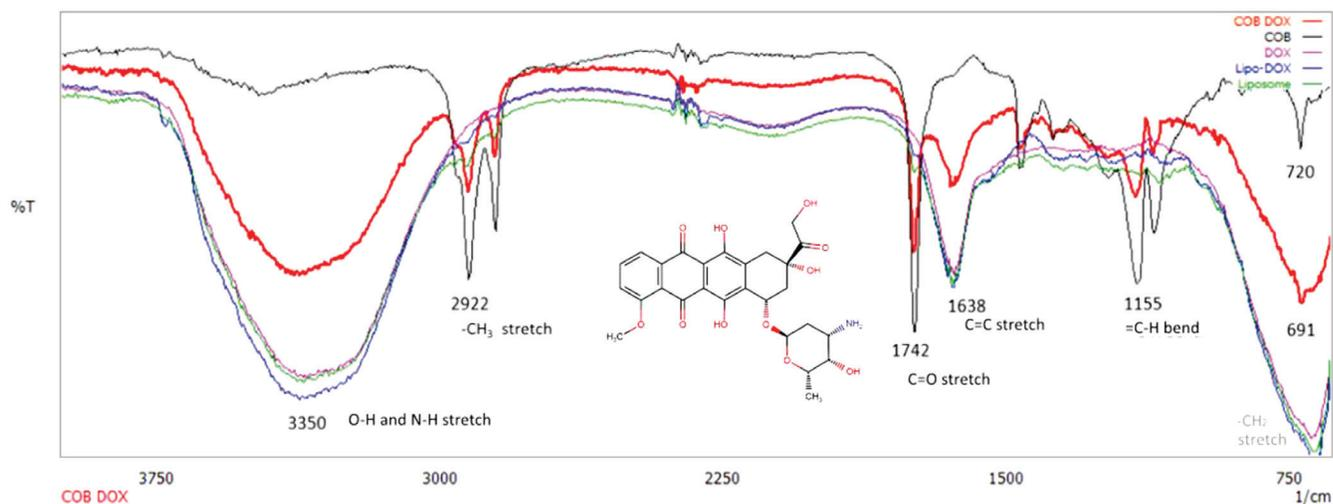
Figure 1. FT-IR absorption spectra DOX-based encapsulation using COB and Liposome.
