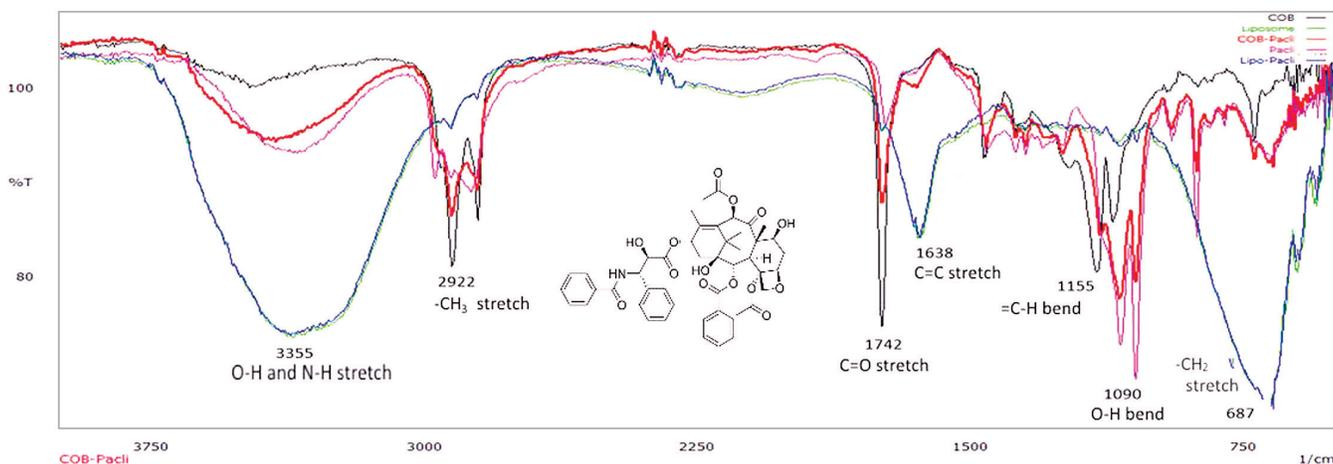
Figure 2. FT-IR absorption spectra PTX-based encapsulation using COB and Liposome.
