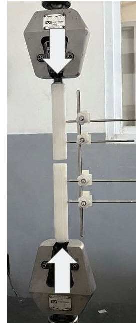
Figure 3. Direction of applied axial load in the fixator system.
